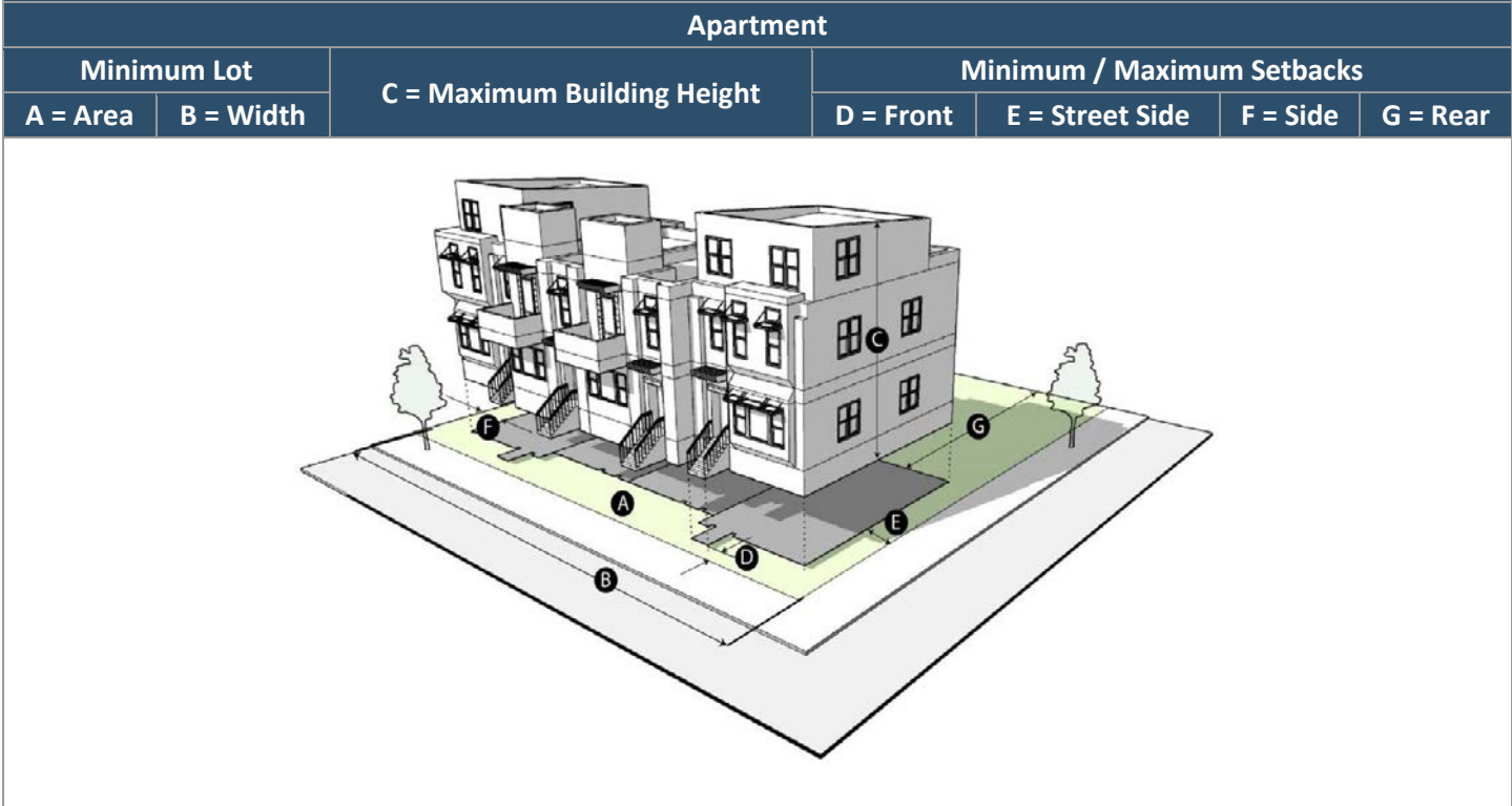
Figure 156.B.004-6 Housing and Building Type Illustrations
