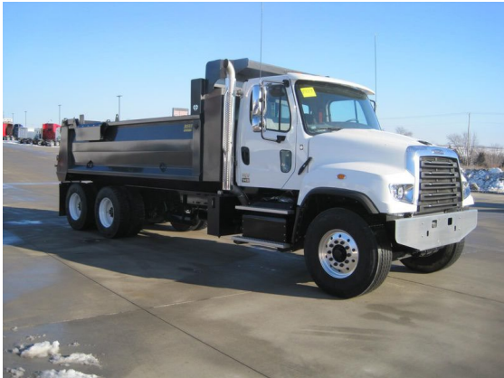
Large Dump Truck (Tandem Axle) - $75, $105.4 FLS = 5.5'W * 16'L * 3.5'H + 2' Pile ~ 13.6 CY
