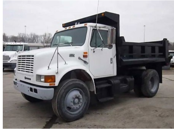
Medium Dump Truck (Single Axle) - $50, $51.93 FLS = 5'W * 10'L * 3'H + 2' Pile ~ 6.7 CY
