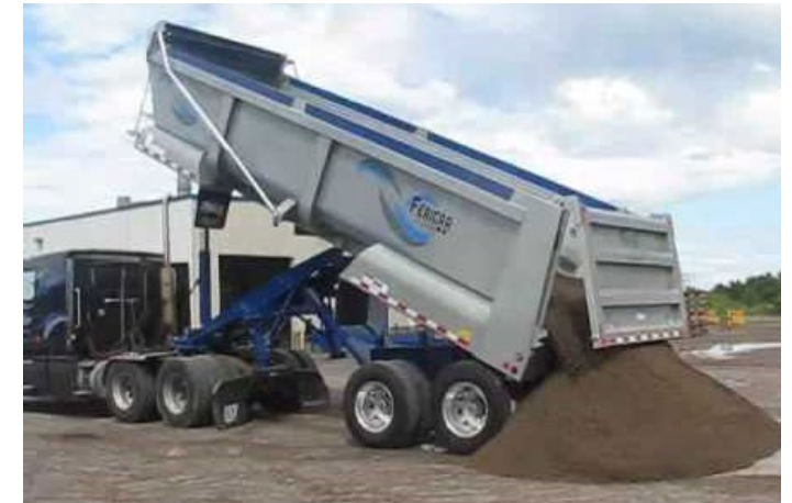
Semi-Truck & Trailer - $150, $179.03 FLS = 6.5'W * 16'L * 5'H + 3' Pile ~ 23.1 CY
