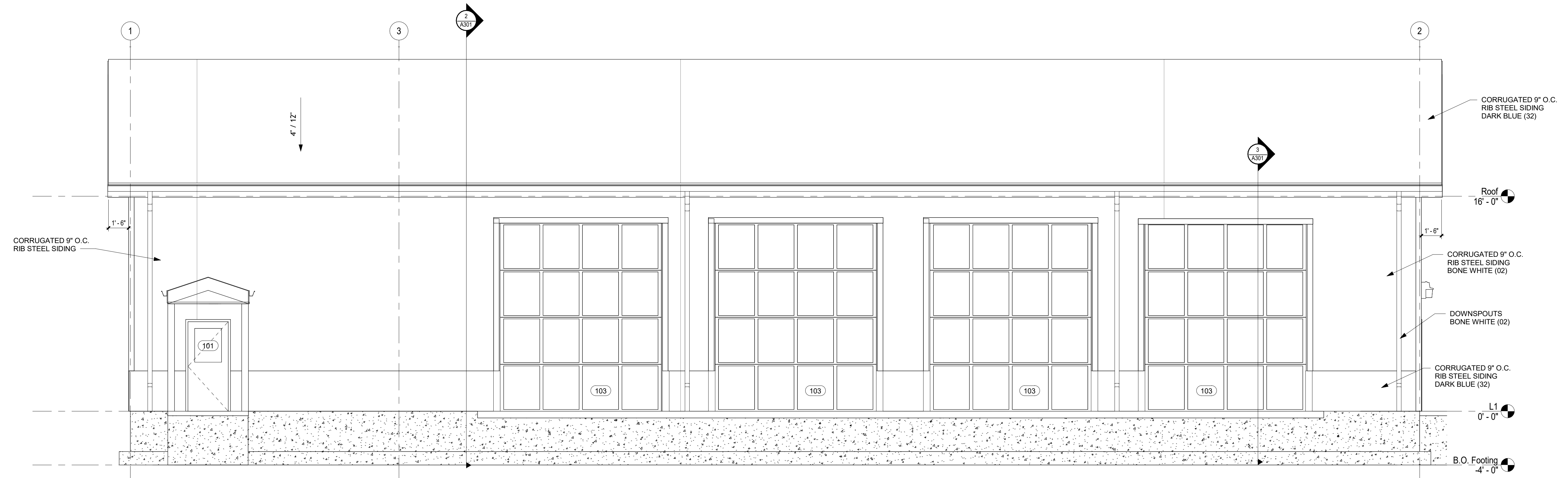
1 South Architectural Building Elevation SCALE: 1/4" = 1'-0"
